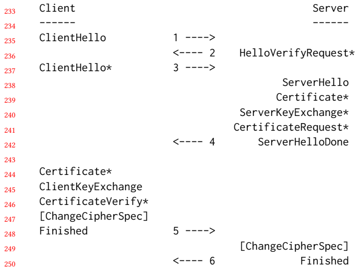
Figure 2: Messages for the full DTLS 1.2 handshake. Optional messages are indicated with an asterisk.
